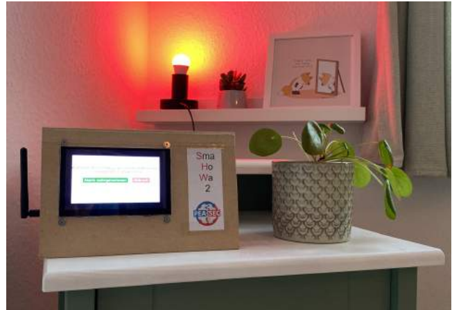
Figure 2: Prototype in study condition showing an alarm on the touchscreen in addition to different visual (white, blue, red light flashing or static) and auditory (siren sound or beeping) stimuli as well as possible smartphone notifications (not shown in this image). The prototype and the light bulb are connected via Zigbee protocol.
